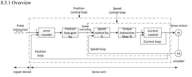
Position control loop diagram (turn off the model loop)
