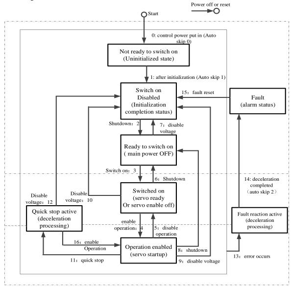
After migrating to operation enabled (after servo enable turned on), lift it to more than 100ms and input the action command.
