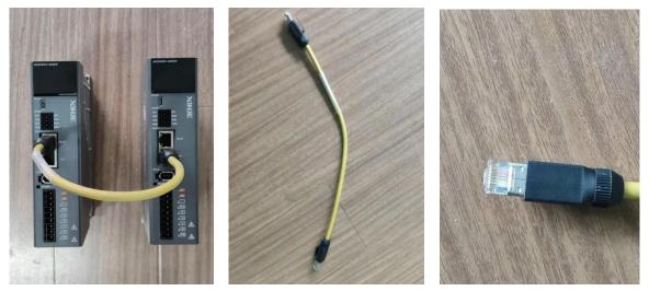
CANopen communication follows the rules of bottom in and top out. For the definition of network cable interface pin, see the terminal description of CN1 in chapter 3.2.
