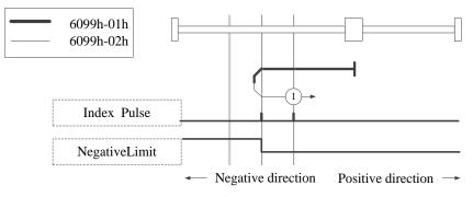
Homing on negative limit switch and index pulse
