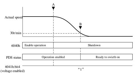
Note: 6041h: bit4 (statusword: voltage enabled) is still 1 and does not change.
