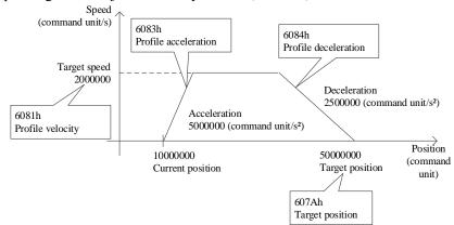
The relative mode or absolute mode can be determined by bit6 (absolute / relative) of 6040h (control word). Action 1: basic set-point
