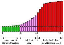
Flexible structure large load: refers to the type of synchronous belt structure, large load inertia equipment. High rigid load: refers to the mechanism of screw rod or direct connection, and equipment with strong mechanical rigidity.
