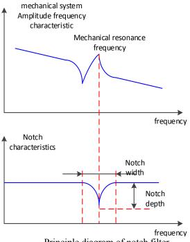
Principle diagram of notch filter
