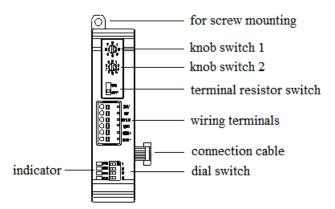
Knob switches 1 and 2 are used to set the node address (i.e. station number) of XD-COBOX-ED module in CANopen network.
